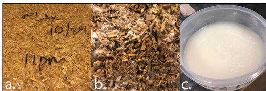
Figure 2. Raw materials to make mycelium-composite: a. Flax, b. hemp, c. flour and water
