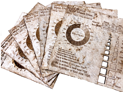
Figure 4. Mycocard test cards laser cut in different thicknesses.
