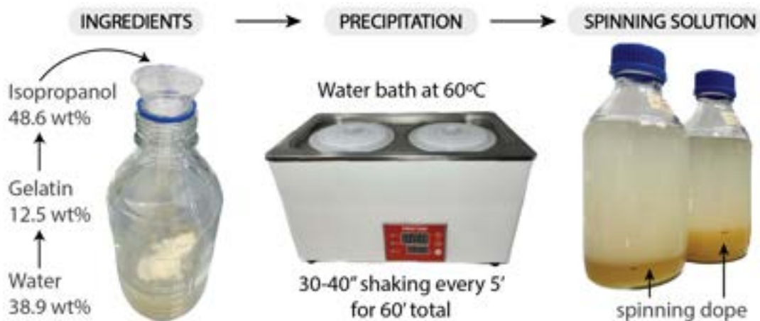
Figure 7: Spinning solution formula and preparation process to obtain spinning solution
