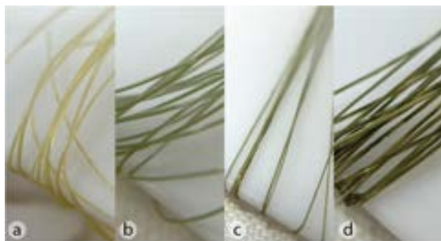
Figure 10: (a-d) Gelatin biofibers change color from light to dark green as the genipin content in its material formula increases in the following increments: (a) no genipin; (b) 0.12 wt% genipin; (c) 0.18 wt% genipin; (d) 0.24 wt% genipin.
