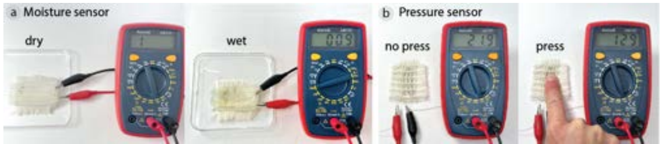
Figure 14: Woven textile sensors with biofibers integrated into the cloth: a. moisture sensor and b. pressure sensor.
