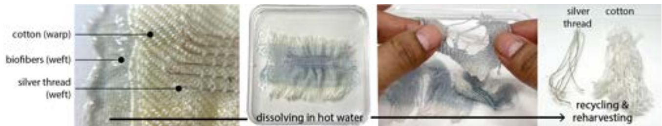
Figure 15: Dissolving biofibers in our woven moisture sensor enables reharvesting of conductive and non-conductive threads at the end of the sensor’s life. This process also applies to our pressure sensor. The biofibers’ change in color is due to the result of genipin (a crosslinker) in its composition.
