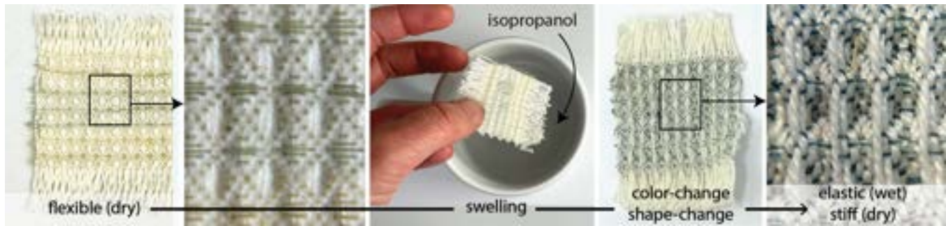
Figure 17: Swelling as an interaction: a woven structure that experiences color- and shape-change due to swelling when exposed to isopropanol.
