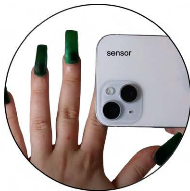
Figure 1: Bio-e-nails are made from a modified form of Alganyl [6]– a biodegradable plastic; the nails embed a Near-Field Communication (NFC) chip that can be programmed for various applications such as navigation; and after use, the bio-e-nails can be composted or recycled for reuse.
