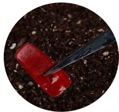
Figure 1: Bio-e-nails are made from a modified form of Alganyl [6]– a biodegradable plastic; the nails embed a Near-Field Communication (NFC) chip that can be programmed for various applications such as navigation; and after use, the bio-e-nails can be composted or recycled for reuse.
