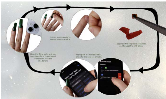
Figure 4: We designed bio-e-nails to be circular: after they are programmed and used, they can be dissembled to harvest the NFC and compost the materials substrate. We experimented with the harvested NFC, and it worked as expected.
