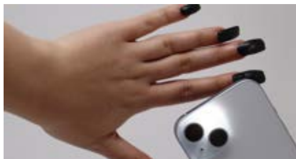
Figure 3: The Bio-e-Nails embed an NFC chip that can be programmed to turn on the phone flashlight.
