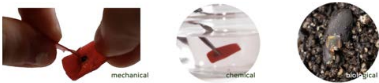
Figure 4: Our interdisciplinary approach enables the exploration of multiple methods for the end-of-life of the Bio-e-Nails. The mechanical method involves separating the layers and pulling out the electronics. The chemical method dissolves the substrate bio-material in water or vinegar. The biological method decomposes the biomaterial substrate in a soil mixture containing micro-organisms. These methods can be combined for a more effective degradation.
