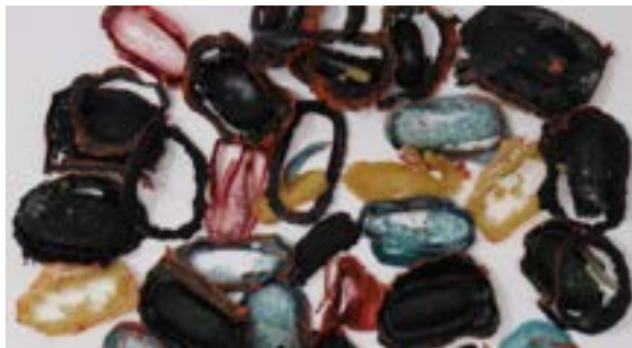
Figure 5: The intermediate versions, considered failure from an aesthetic and functional perspectives, were re-used to create new nails. This was possible because we chose a bio-material that can be reversed from solid to fluid state by adding water and heating them in the microwave.
