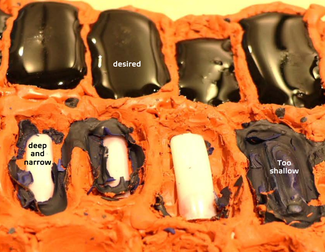
Iterative low-tech fabrication process of Bio-e-Nails using hand-crafted clay wells for chitosan-based nails.
