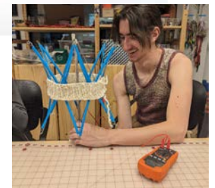
A band knit with MerinoX changes resistance when stretched on an umbrella swift.
