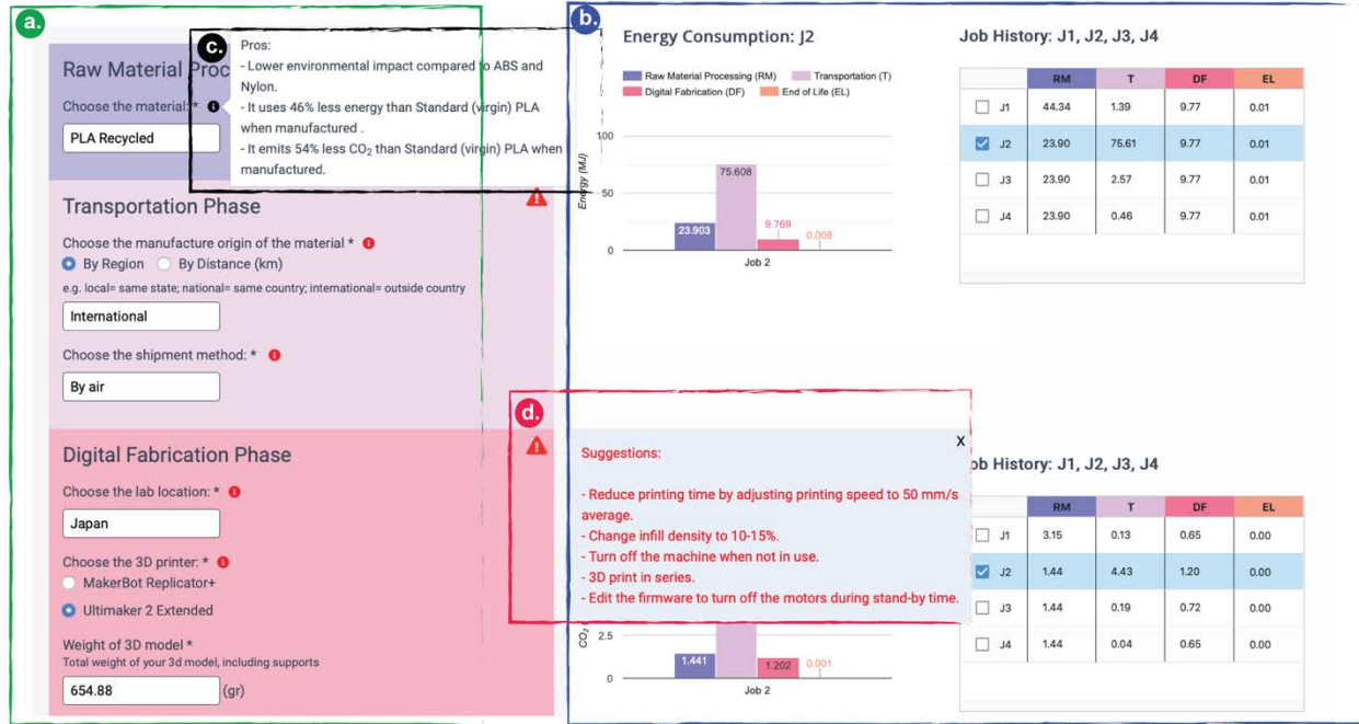
Fig. 2. Yupana Interface. a) User input data, b) bar charts and job history tables showing the energy consumption and CO 2 emissions, c) learning information, and d) sustainability suggestions.
