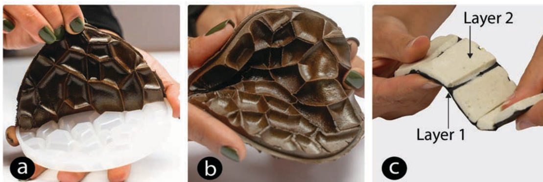
FIGURE 3.11: a. Demolding the biofoam sample. b. Biofoam acts like memory foam, c. Biofoam applied in layers.
