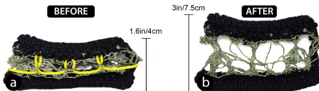
FIGURE 4.5: “Unfolding Lace Top” swatch to test the unfolding stitch structure. a. before, and b. after dissolving the swatch in cold water.
