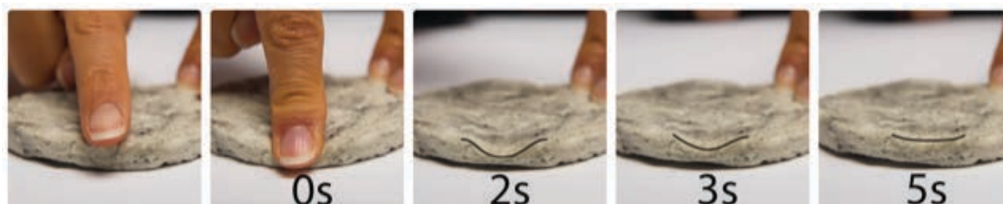
FIGURE 3.6: Conductive biofoam spring back time.
