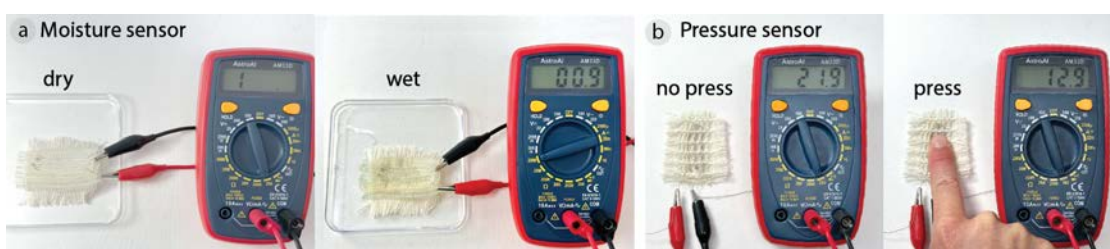
FIGURE 5.14: Woven textile sensors with biofibers integrated into the cloth: a. moisture sensor and b. pressure sensor.
