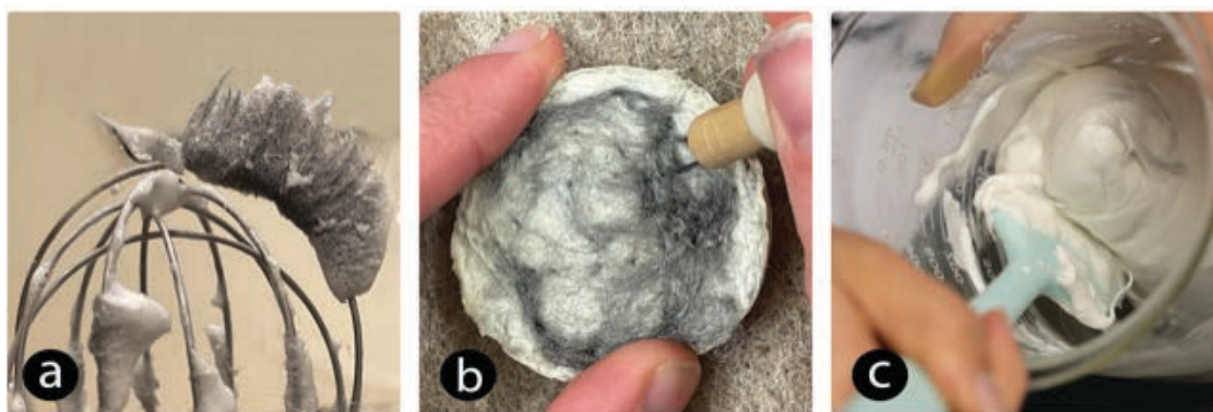
FIGURE 3.3: Attempts to incorporate stainless steel fibers into biofoam: a. whisking, b. felting, c. folding
