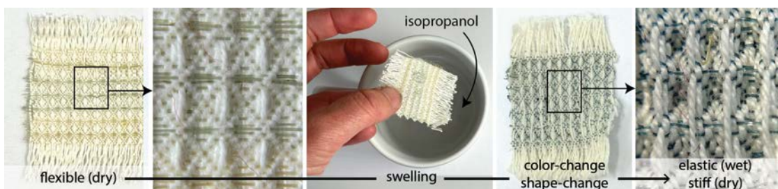
FIGURE 5.17: Swelling as an interaction: a woven structure that experiences color- and shape-change due to swelling when exposed to isopropanol.
